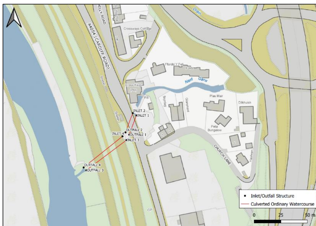
Figure 8: The Nant Garw culverted ordinary watercourse which runs beneath the A4054 Cardiff Road
