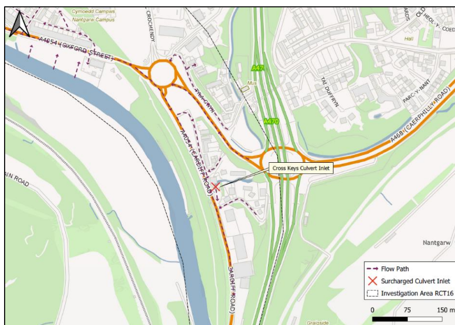
Figure 7: Indicative flow paths observed during Storm Dennis to the south of RCT16
